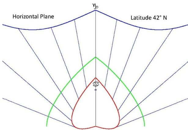
Fig. 29 Craticle at latitude 42 with elliptical gnomon
