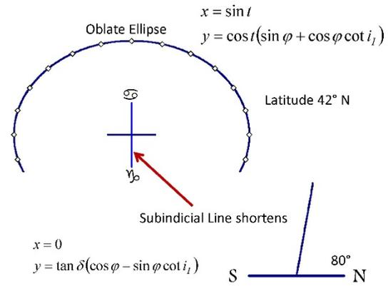
Fig. 5 Elliptical Sundial – Inclining Index
