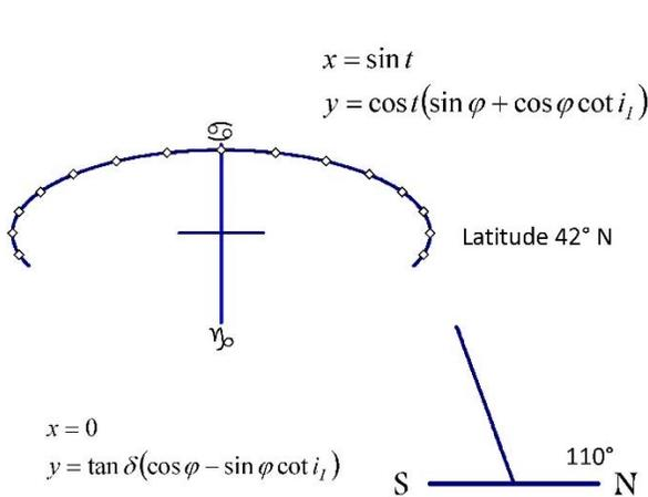
Fig. 15 Inclining the index to the South
