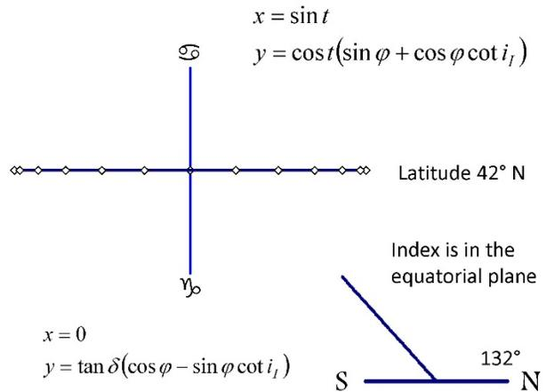
Fig. 16 Foster's Diametral Retrograde Dial
