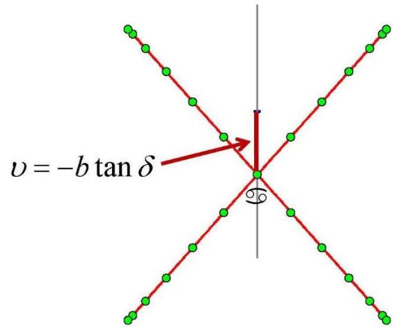
Fig 36 Equation for the declination adjustment form
