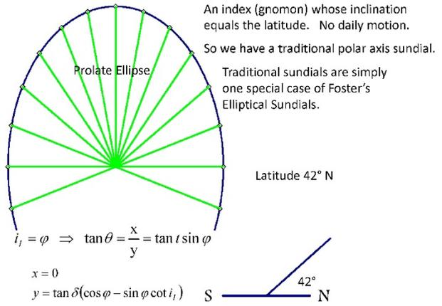
Fig. 7 Elliptic Dial with Index Parallel to Polar Axis
